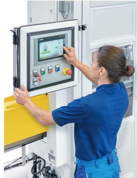
Simple operation of the PLC via an HMI touch panel
